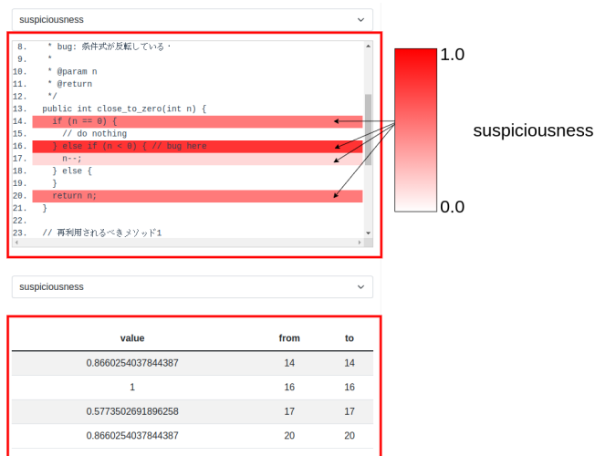
Figure 1. Proposed method to visualize the suspiciousness values in the detailed information of the variant
