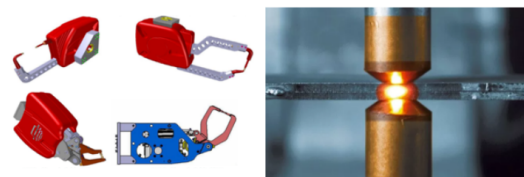
Figure 1: Example of welding guns (left) The union of two pieces of metal through spot weld (right)
