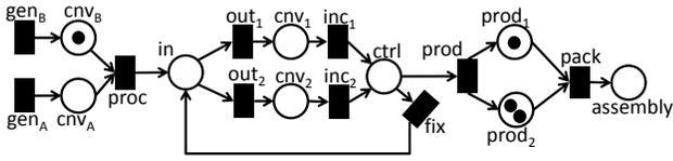
**Figure 2. Petri net modelling an assembly line.**
