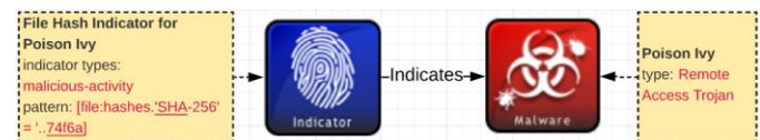
Figure 1. A simple indicator uses a file hash to indicate the presence of Poison Ivy
