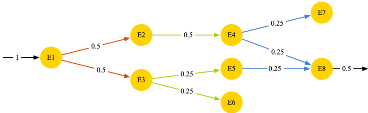
Fig. 2. An example for calculating relation path’s reliability. Entities are represented by yellow dots and numbered from 1 to 8. Three kinds of relation r_1, r_2 and r_3 are displayed with red, green and blue arrows, respectively. When calculating the reliability of the relation path p = (r_1, r_2, r_3) between E_1 and E_8 , we assign 1 unit of resource to E_1 and make the resource flow along the graph. Finally, we’ll obtain 0.5 unit of resource at E_8 , which means the reliability of p is 0.5.
