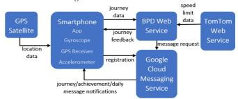
Fig. 1. BackPocketDriver component diagram
