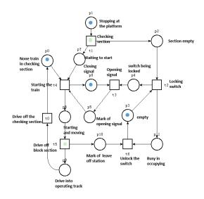
A pivotal difference of IROM compared with ROM is that the train's position checking results of protection system play as a key precondition to start next train. In this case, IROM prevents train from start when signal machine turn to green once any signal equipment fail to work. It is pointed out that the checking system is very useful when signal system converts to degraded mode.
