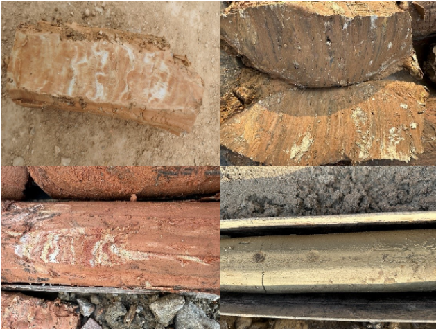
Figure 8: Examples of silty clay drill cores with diverse colors and textures.
