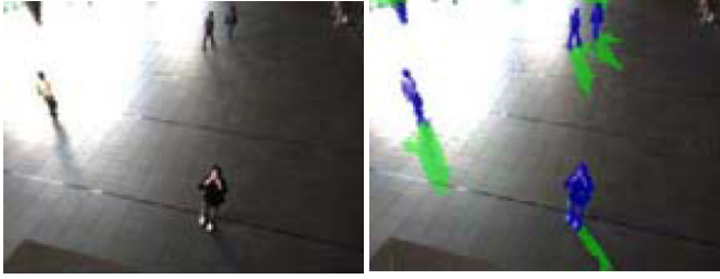
Figure 5. In this figure an example of shadow detection performed with the proposed algorithm for an out-door environment is reported. Shadow pixels are represented in green.
