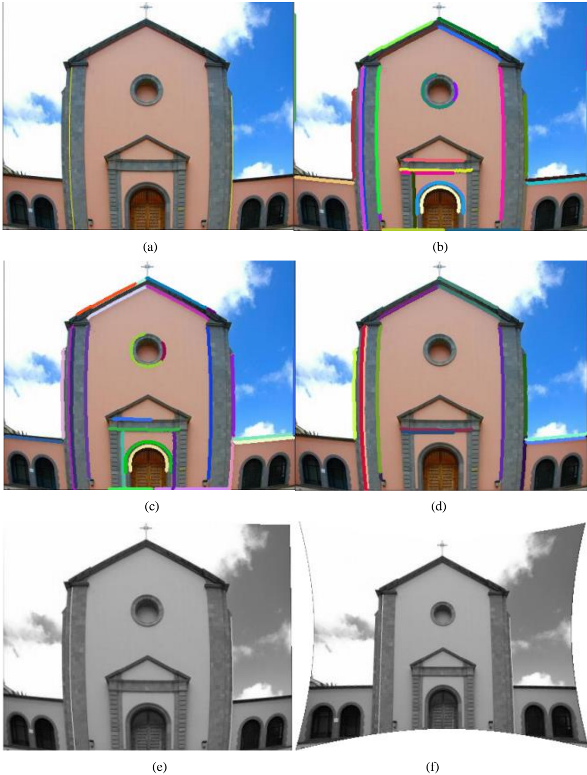
Figure 7. Lens distortion correction for a real image:(a) Original image, (b) detected candidate arcs, (c) choose the good arcs using the Bukhari-Dailey method, (d) choose the good arcs using the proposed method, (e) undistorted image using the Bukhari-Dailey method, and (f) undistorted image using the proposed method.
