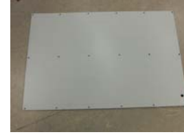
Figure 6. IR-emitting board (before being coated with aluminum foil) that we developed for our prototype of SyncSurface Table.
